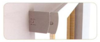
4. When all brackets have been fitted insert blind by lining up fascia end caps with slots on fixing brackets. Adjustment of fascia end caps can be used to aid this process. When both sides have been located ensure blind is pushed fully home until locks on both the fixing brackets and centre support have been snapped in to place.
