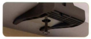
3. Keeping the tool in place, either drill a pilot hole through the centre of the holes on the bracket, or - if fitting to a suitable substrate - directly drive a screw up into the recess until tight. Ensure the tool stays flat and square against the recess while doing this. Once the screw is tight, the tool can be pulled out of the bracket. NOTE: The use of wall plugs is recommended where appropriate.
