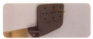
Pick the required overlap: 22mm (marked 'recess fit'), 50mm or 765mm. Keeping the tool in place, drill into the fitting surface using a 3mm bit through 2 of the 4 grouped holes. Where centre support is required, position tool in centre of window and drill required holes. It is recommended to use the top and bottom holes where possible.
