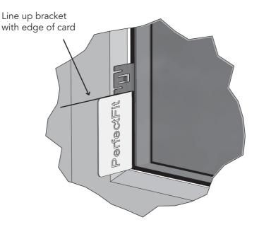
Line up the bracket with the base or top of the credit card (depending on which corner of the window you are working) and fit the bracket by pushing it between the glass and the rubber seal of the window.
