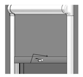
To lock the blind into position, rock the handle backwards.
