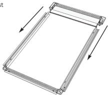
Fix securely with the two screws on each joint.
