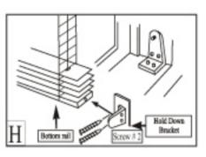
Hold down brackets: Using two small screws, screw hold down bracket to window facing or wall. Snap bracket pin ends into the hole at bottom rail end.
