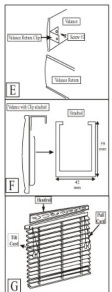
For Outside Mount: Screw one end of the valance return clip onto the valance using Screw #3. Align the edge of the valance return with the valance. Screw the other end of the valance return clip onto the valance return.
