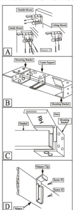
Brackets should be placed at the width of blind's head rail 6mm past each end. The bracket doesn't necessarily need to touch the inside face of the window frame.
