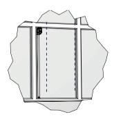
Bead depth can be measured using a depth gauge. This gives you the measurement from the face of the window frame to the glass.
